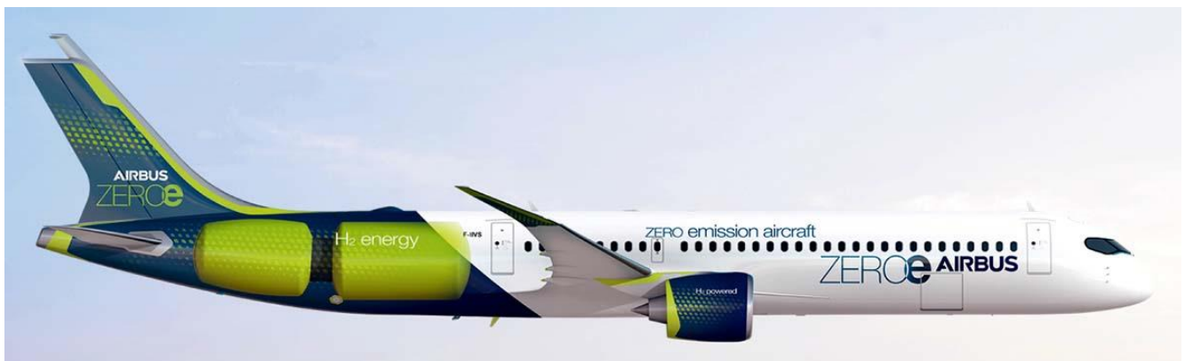
Figure 5. How to store liquid hydrogen for zero-emission flight. Source: Airbus.
